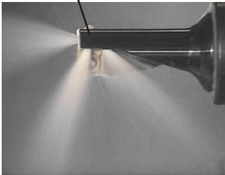
EcoCut offers an innovative detail solution for range 2.25D, namely additional bidirectional coolant supply for better chip evacuation.
