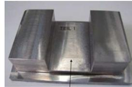
Result: Workpieces with clean surface, close tolerances and reduced formation of burrs, maximum service life of tool and insert.
